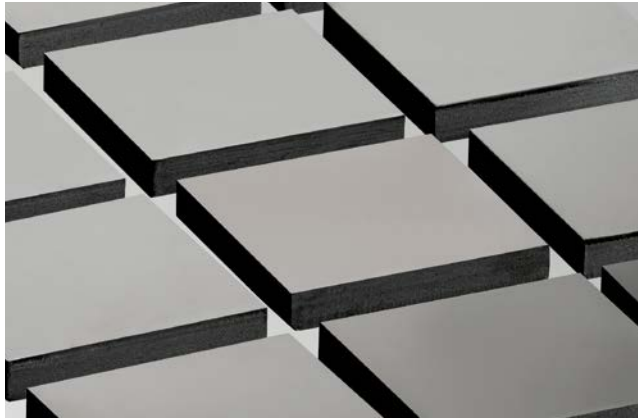
Precise dicing of a silicon wafer.
