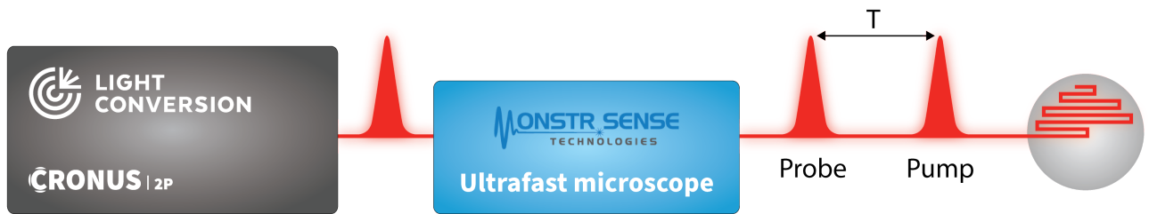
Figure 1: Schematic of the setup: Laser beams from the Light Conversion's CRONUS-2P femtosecond laser enter the MONSTR Sense Technologies' ultrafast microscope, composed of a BIGFOOT® and NESSIE® system. Within MONSTR Sense's ultrafast microscope, pump and probe pulses are generated and raster-scanned across the sample using a combination of Galvo and wafer-stage scanning.
